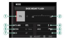
To prevent the built-in flash firing when a shoe-mounted flash unit is attached, select **OFF** for **I FLASH SETTING** > **Built-In Flash**.
