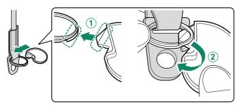
Place a protective cover over the eyelet as shown.
