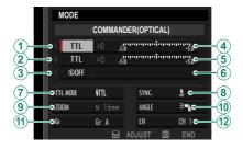
Fujifilm optical wireless remote flash control offers a choice of four channels (Channels 1 through 4) for the exchange of optical signals between the commander and remote flash units. Separate channels can be used for different flash systems or to prevent interference when multiple systems are operating in close proximity.
