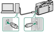
USB connector (Type-C) Leave the computer on during charging.
